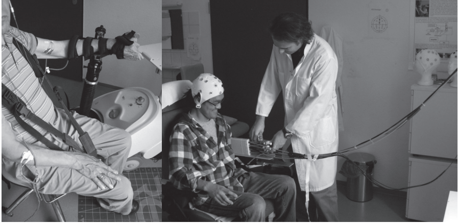
Figure 1. Stroke Rehabilitation BMI Experimental Setup: Left panel: patient controlling the reach and grasp movement of his paretic limb using the EEG-based BMI system. On the right Dr. Ramos-Murguialday adjusting the robotic orthosis hand to be controlled by means of an EEG-BMI by the user.
